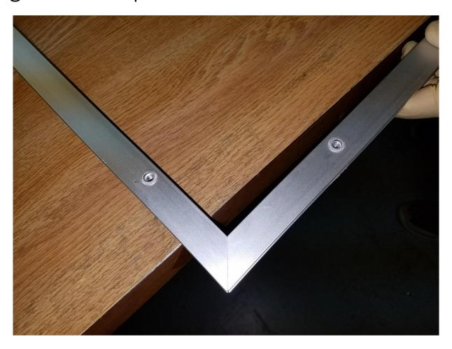
Depending on the size of the screen, one or more "stiffening' members will be required to allow the screen to hold tolerance. Hole-to-hole tolerance on the inserts is +/- 1/16" The inserts can be strategically located to miss key components in the minienvironment, where required.
